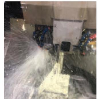
Machining with oil filtered to one micron with the Transor
